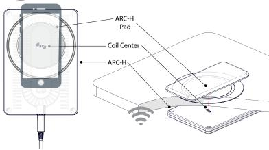
The ARC logo identifies the coil center which must be aligned with the resonator pad
