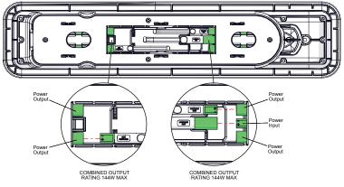
\*SIT STAND MECHANISM CAN BE CONNECTED TO EITHER END OF THE BATTERY BUT NO CONNECTIONS MUST BE MADE TO THE 2ND OUTPUT
