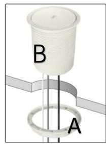
4. Tighten the fixing ring (A) against the worktop.
