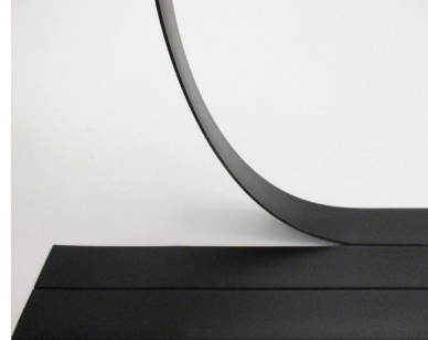
Removal of excess material on the pre-scored line
